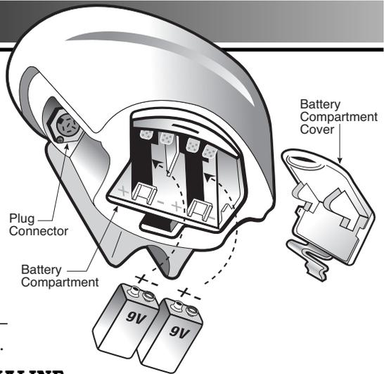
Most metal detector problems are due to improperly installed batteries, or the use of non-alkaline or discharged batteries. **If the detector does not turn on, please check the batteries.** Batteries shall be disposed of in a safe way. Only dispose of batteries in specific collection containers (contact your retailer for more information) in order to protect the environment
