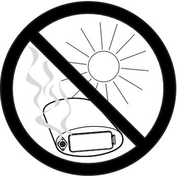
Use and store the metal detector only in normal temperature environments. Extreme temperatures can shorten the life of electronic devices and distort or melt plastic parts.
