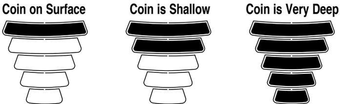
Objects other than coins will still register on the 5-segment depth scale, but the depth indication will be relative. For example, all 5 bars illuminated could indicate a coin buried 9" deep, but could also be a very large object several feet deep. Use the Depth Indicator in conjunction with the Target-ID system and the aid of Pinpoint to gain more information about a buried target.
