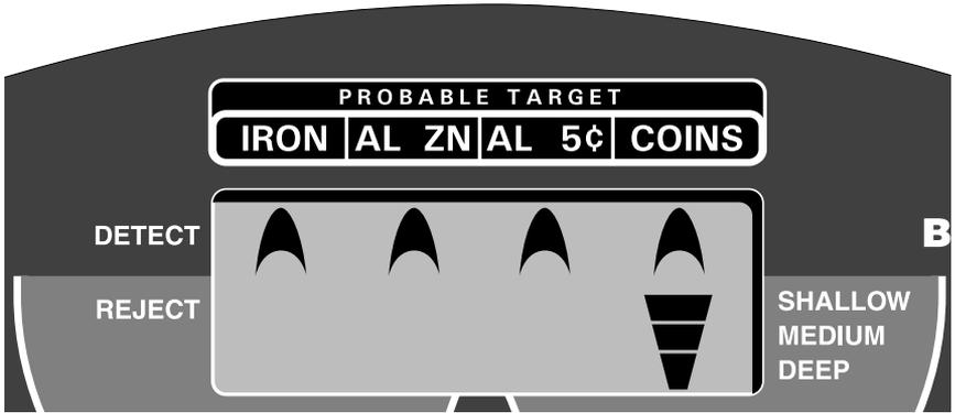
The four categories depicted across the top of the display indicate the probable identification of buried, detected metal objects. The searchcoil must be in motion over an object to be detected. Alternatively, you can pass an object over a motion less searchcoil to test your detector. One of the four target indicators will illuminate, indicating the probable identification of the object. The indicator will remain illuminated until another object is detected.
