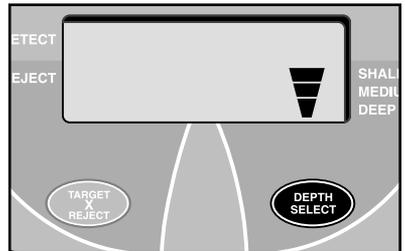
When three segments are illuminated, the detector is at maximum sensitivity. As you press the DEPTH SELECT touch pad, the detector toggles among the three different sensitivity levels. A more detailed explanation of depth selection is found on page 14.
