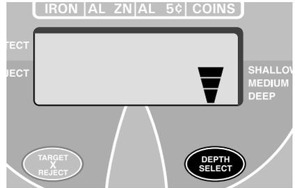
At the maximum depth setting, the detector will detect a coin-sized object buried approximately 6 1/2 inches beneath the surface. With two depth segments illuminated, the detector's depth range will be reduced to 80%, and with one depth segment illuminated, the range will be reduced to 65%.
