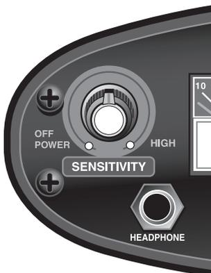
Sensitivity will be reduced slightly when using the Tracker IV in the Tone Discrimination mode. If you want optimal depth capability, operate in the All Metal mode by turning the Discriminate control completely counterclockwise; then turn the Sensitivity control clockwise to its highest clockwise position without chatter. If your Tracker IV chatters or beeps erratically, reduce the Sensitivity by turning the left knob counterclockwise.
