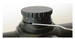
3. Keeping firm grip on the knob, use the pen to turn the dial back to zero, lining up the number zero with the white indicator dot. Only the numbered dial should move – do not allow the entire knob to move or else you will alter your windage and elevation zero settings.
