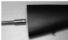
3. Place the SpeedBead **plate** with pins forward against the receiver making sure that the pins begin engagement into receiver holes.
