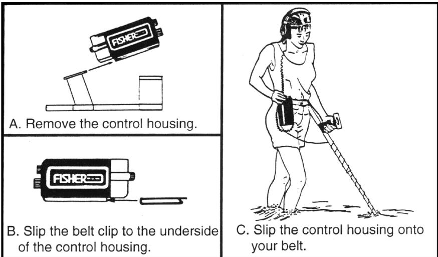
Figure 3. You can hipmount your 1280-X by sliding the control housing from the handle and attaching it to your belt. This reduces the weight of the stem, creating nearly effortless hunting.
