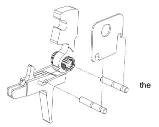
\*Installation of pin keeper shown
