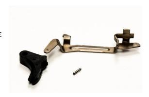
7. USE A .050 ALLEN KEY TO REMOVE THE THREADED PIN ON THE KILLER INNOVATIONS TRIGGER SHOE. PLACE A SMALL AMOUNT OF BLUE THREAD LOCKER ONTO THE THREADED PIN. SLIDE THE SHOE ONTO THE TRIGGER BAR AND THREAD THE PIN INTO THE HOLE. TIGHTEN THE THREADED PIN DOWN HAND TIGHT.
