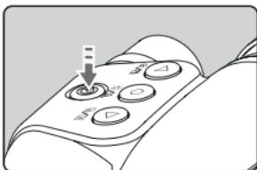
Press and hold <
