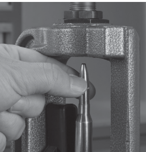
Place a bullet on top of the primed and powder-charged case.
