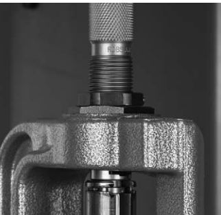
Steel Sizer Die adjusted to contact Shell Holder.
