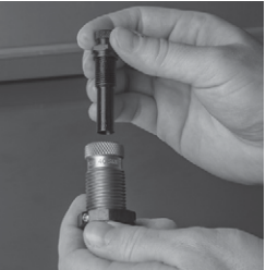
Most Seater Dies in our three-die sets use a “through-the-top” style Seater Plug, as shown in this photo. This allows for easy cleaning.
