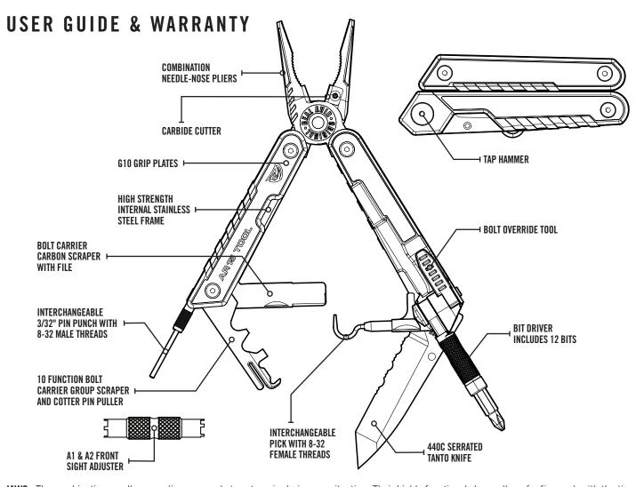
**JAWS:** The combination needle-nose pliers are made to get a grip during any situation. Their highly functional shape allows for fine work with the tip as well as bigger, more aggressive tasks towards the back of the jaws. The carbide cutter is designed to cut most common gauges of copper wire.
