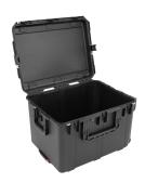
SKB iSeries Injection Molded Mil-Standard Waterproof Cases are molded of ultra high-strength polypropylene copolymer resin, featuring a gasket-sealed, water and dust tight, submersible design (MIL-STD 810H) that is resistant to corrosion and impact damage.
