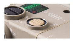
Integrated Push-Button Activation and remote cable-pressure-pad switch activation; tap and release for momentary activation; tap twice for 5-minute continuous ON.
