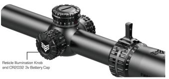
The reticle illumination knob is located on the left side of the scope body. Unscrew the battery compartment cap counter-clockwise and insert the CR2032 3V battery with the + side facing outwards and the - side facing the scope body. Carefully screw the battery cap back into place finger tight, taking care not to cross-thread it.
