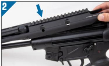
Place the upper half of the handguard over the top of the receiver making sure the charging handle passes through and the receiver's claw mount interface is aligned with the handguard's corresponding mounting holes. There are four mounting holes, two on the left and two on the right side of the handguard.
