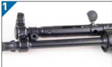
Remove the handguard and handguard retainer pin. Lock charging handle to the rear in its locking recess notch.
