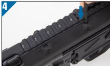
Thread the four pan-headed T10 screws into the locking lugs. Once threaded, proceed to tighten each screw evenly by alternating between them using the included T10 wrench.
