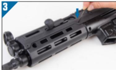
Thread the four flat-headed T10 screws. Once threaded, proceed to tighten each screw evenly.
