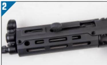
Insert the lower half of the handguard upwards from below the barrel. Align its threaded screw holes with that of the countersunk holes in the upper half of the handguard. This may be a tight fit and some resistance may be encountered.
