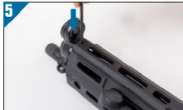
Thread the included brass-tipped set screw into the corresponding threaded hole located on the top of the handguard and just behind the front sight. Using the included T10 wrench, tighten the set screw until it makes contact with the cocking tube. (Do not over tighten)
