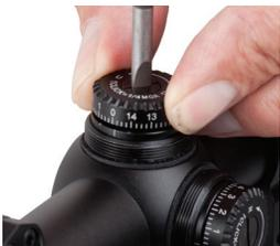
3. Install dial and reinstall and tighten center screw while firmly holding the dial..
