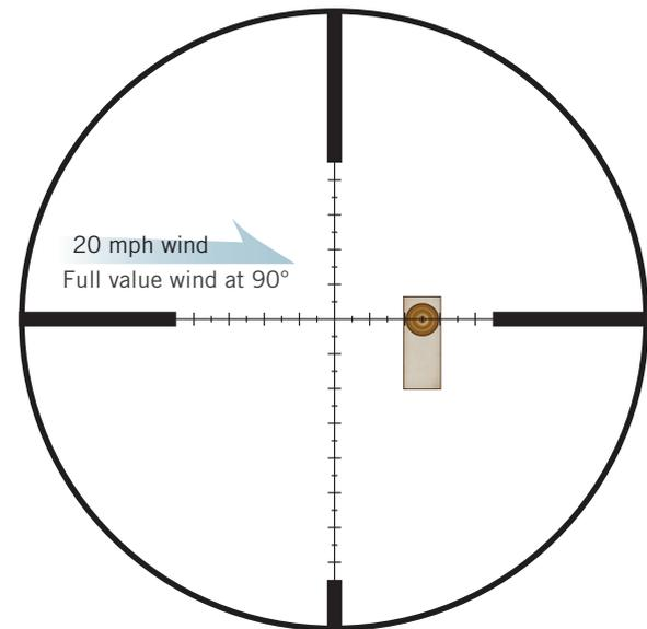
10 MOA reticle correction for 20 mph wind at 700 yards. Elevation is already dialed into turret.
