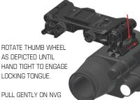
PULL GENTLY ON NVG TO ENSURE THAT IT IS SECURELY ATTACHED.
