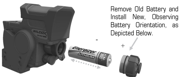
Figure 4.2-2 Replacing the Battery in the RAAM GSS
