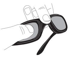
2) Rotate the gasket up to engage the corresponding slot and tab at the top of the hybrid.
